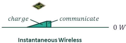
Figure 10. Minimal power usage of iW facilitates passive tags.
